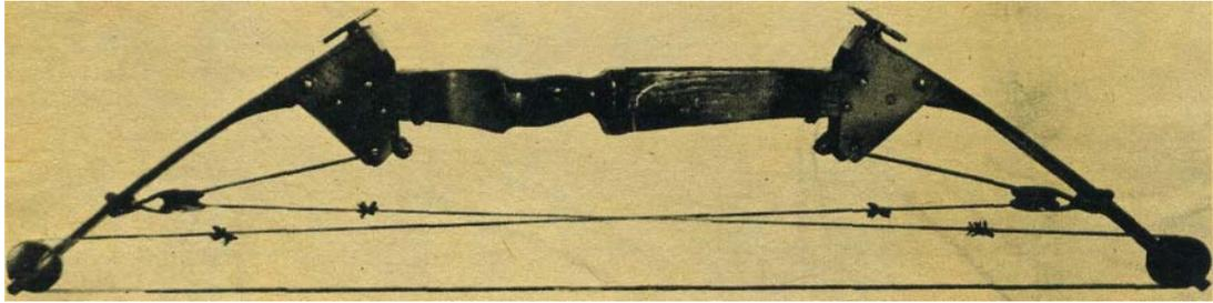
*Bow string rolls over eccentric wheels at ends of compound bow, dropping the pull to ease strain on archer.*
